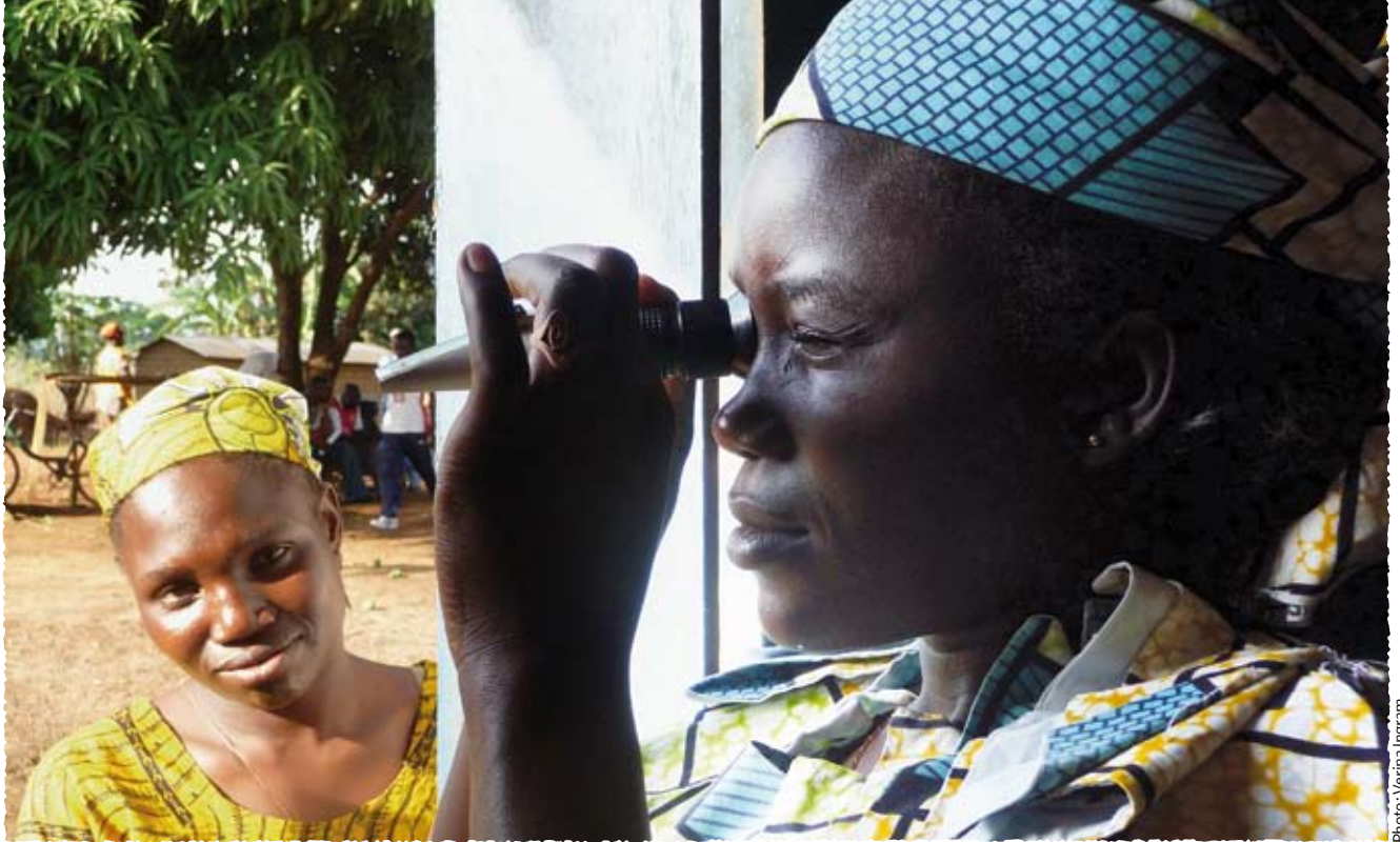
Aminatou Hamoua, Guiding Hope's internal control officer, uses a refractometer to measure moisture content in honey, ensuring its quality.
