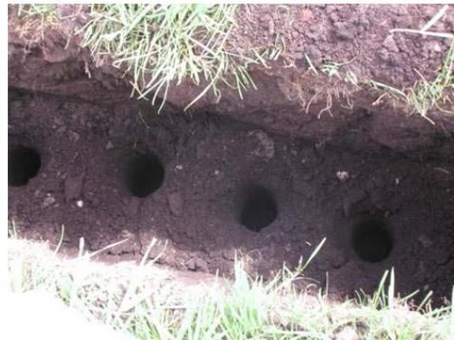
*Figure 3. Soil samples at depths of more than 30 cm were taken using a special soil sampler.*
