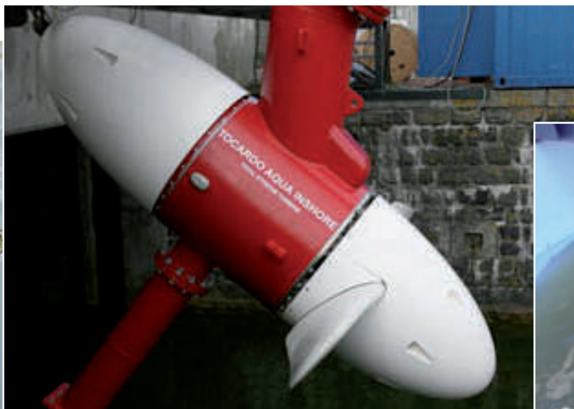
Boven: Tocardo turbine van Teamwork Technology in de spuilsuis.
