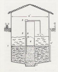
1 = water level 2 = well, concrete rings 3 = motor 4 = methane gas holder
