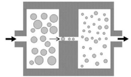
Microfluidic method developed to measure interfacial tension
