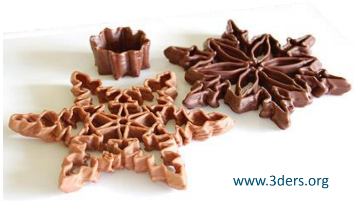
Fused deposition modelling of chocolate (paste)
