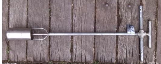
Figure 7: auger used to take potato root samples
