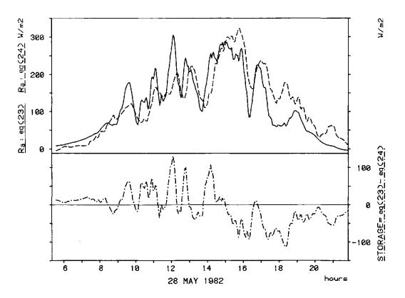
Fig. 2 Radiation absorbed by the canopy during a spring day, with scatteredcloudiness, as calculated by eqs (23) and (24) with G = 0, respectively The difference between the two estimates (interpreted as the storage of heat, see text) is shown at the bottom. Line types used are shown below the corresponding names which appear alongside the scale to which they have to be referred
