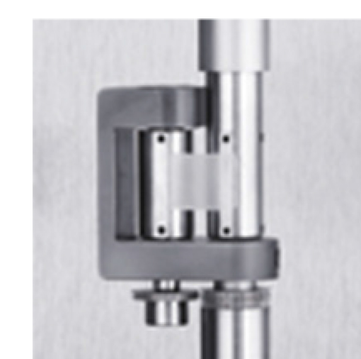
Figure 3. Rotational rheometer at FBR with extensional viscosity fixture intended to be used for determining shear and extensional viscosity parameters
