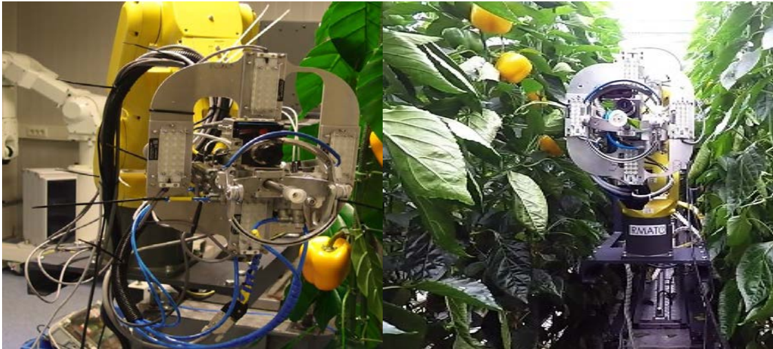
Figure 1: the gripper with the iDS camera, laser and suction cups.
