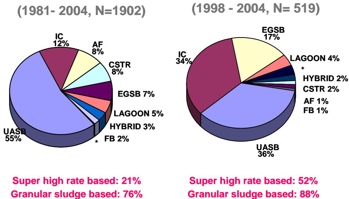
*Figure 1. Implemented anaerobic technologies for industrial wastewater pictured for the period 1981-2004 ( left) and the period 1998-2004 (right). UASB: upflow anaerobic sludge blanket; EGSB: expanded granular sludge bed; Hybrid: combined system with sludge bed at the bottom section and a filter in top; IC: internal circulation reactor; type of EGSB system with biogas-driven hydrodynamics AF: anaerobic filter; FB: fluidized bed reactor; CSTR: continuous stirred tank reactor.*
