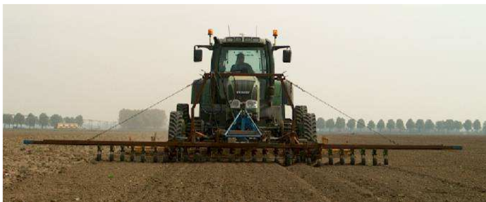
Figure 2. Wide-span tractor with rubber tracks and RTK-DGPS guidance.
