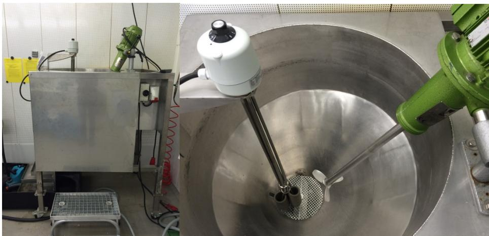
Washing mill (outside and inside) , including heater. Heater is removed before washing process.
