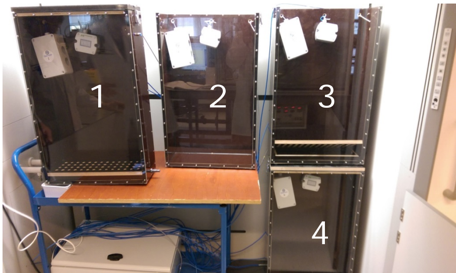
Figure 6 Experimental set-up. From left to right: (1) Ventilated box with rot; (2) Closed box with rot; (3) Ventilated box with healthy potatoes; (4) Closed box with healthy potatoes
