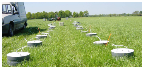
Figure 1. Flux measurements using closed chambers.
