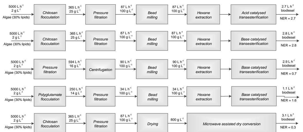
↑ Figure 4. Biodiesel yield and NER for optimised micro-algae to biodiesel process chains, each consisting of other unit operations. The NER is low in path 3 (high energy in first two processes) and path 5 (drying). Biomass losses with non-optimal flocculant dosage decrease also the NER and biodiesel yield.
