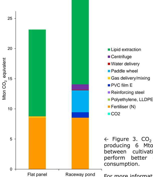
← Figure 3. CO<sub>2</sub> equivalent LCA impact for producing 6 Mton algae oil. Impact vary between cultivation systems. Flat panels perform better due to the lower water consumption.
