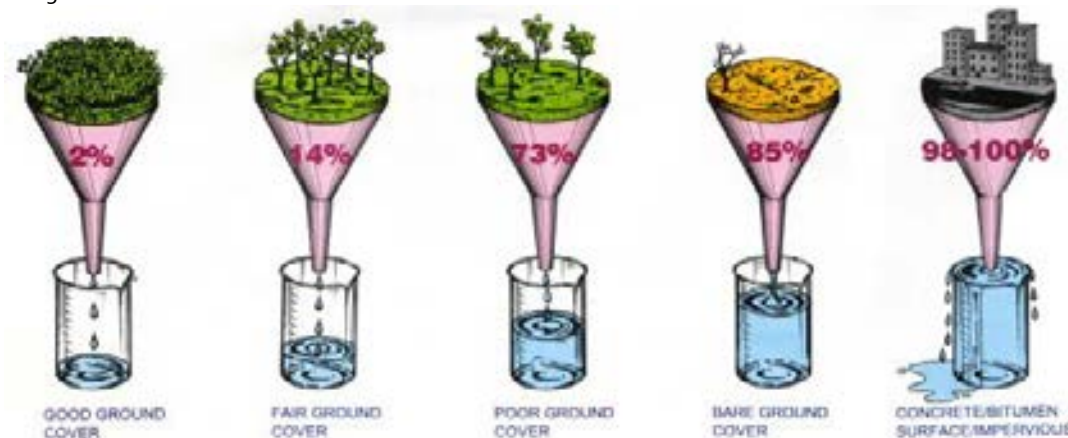
Figure 1.16 Natural surfaces allow water to infiltrate into the ground, less surface runoff is created. While the percentages of paved surfaces occur in the urban area, the groundwater recharge process is prevented, resulting in more runoff. Source: Upper Parramatta River Catchment Trust, 2001.
