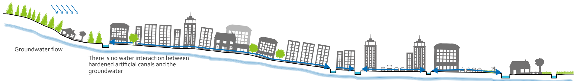
Fig 1.14. During the urbanization, low-lying natural and rural areas are converted into urban areas, paved surfaces prevent create more surface runoff, while streams are either buried or canalized.
