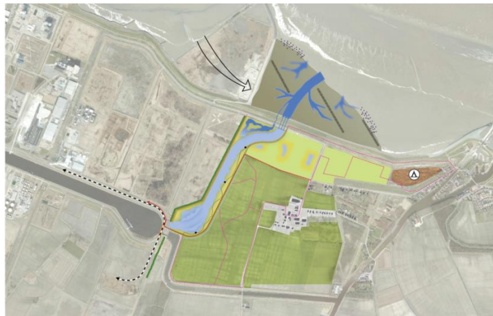
Figure 6. Proposed design of the fresh water outflow at Delfzijl including the development of an estuarine gradient with marshes (Verhoogt et al, 2014).
