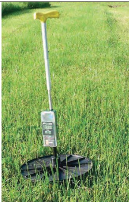
The availability of grass on Rod MacBean's unit is measured using a plate meter
