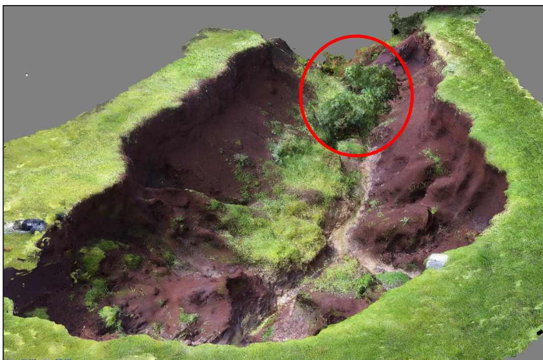
Figure 27: Looking from the gully head to gully exit, and example of the representation of vegetation in a 3d model. The bushes (circled) in "Waterfall" gully are part of the surface.
