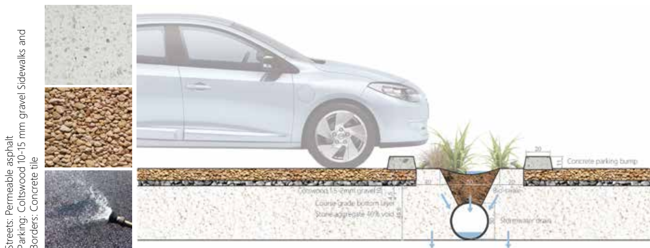
Figure 11.15 Cross section of the innovative technique and materials that ensure large amount of water can be soaked into the ground
