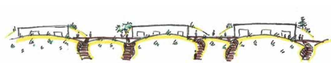
Figure 11.33 Principle sketch of wooden dune structures that function as dune crossings and support dune formation
