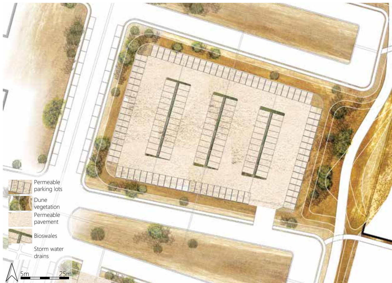
Figure 11.12 Plan of a parking lot with permeable materials, designed as urban flood plain
