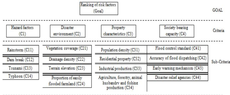
Fig. 4 Triangular fuzzy AHP hierarchical structure
