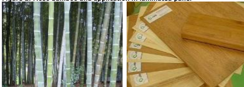
Figure 2: Moso bamboo and application in laminated panel
