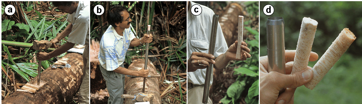
Figure 7.2 Taking trunk pith samples from a felled sago palm: a. the auger is hammered into the pith through a window opened in the wa'ah . b. the pith sample is pushed out of the auger with a wooden stick. c. auger and intact pith sample. d. close-up of business end of auger and of pith sample broken in two.
