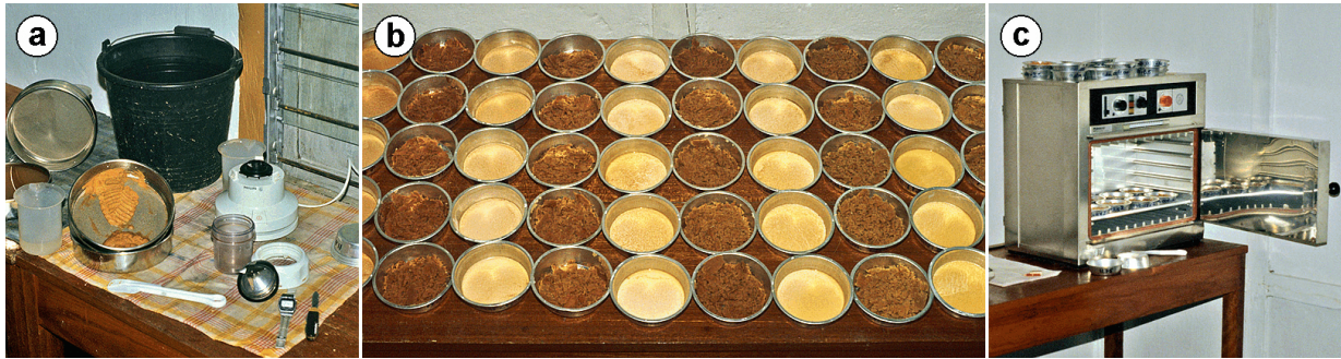
Figure 7.4 Separation and drying of starch and other non-water-soluble solids in sago palm pith samples: a. kitchen blender, and 150-micron-mesh soil sieve with partly separated ground pith sample; b. aluminium dishes with separated starch (whitish) and other non-water-soluble solids (brown) before drying; c. drying cabinet.
