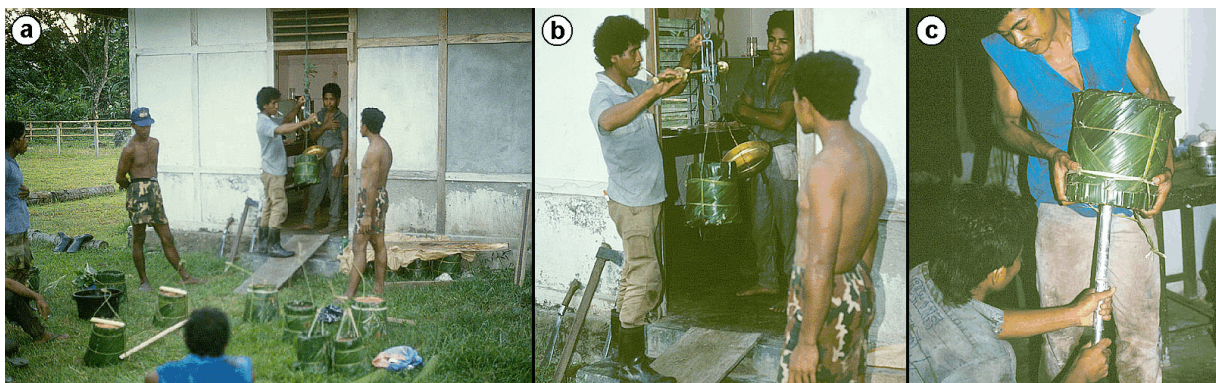
Figure 7.14 Weighing the tumang and drawing a wet starch sample from it. [photo nrs. 90.11-149-02, -03, -04, Hatusua, West Seram wed21nov1990]
