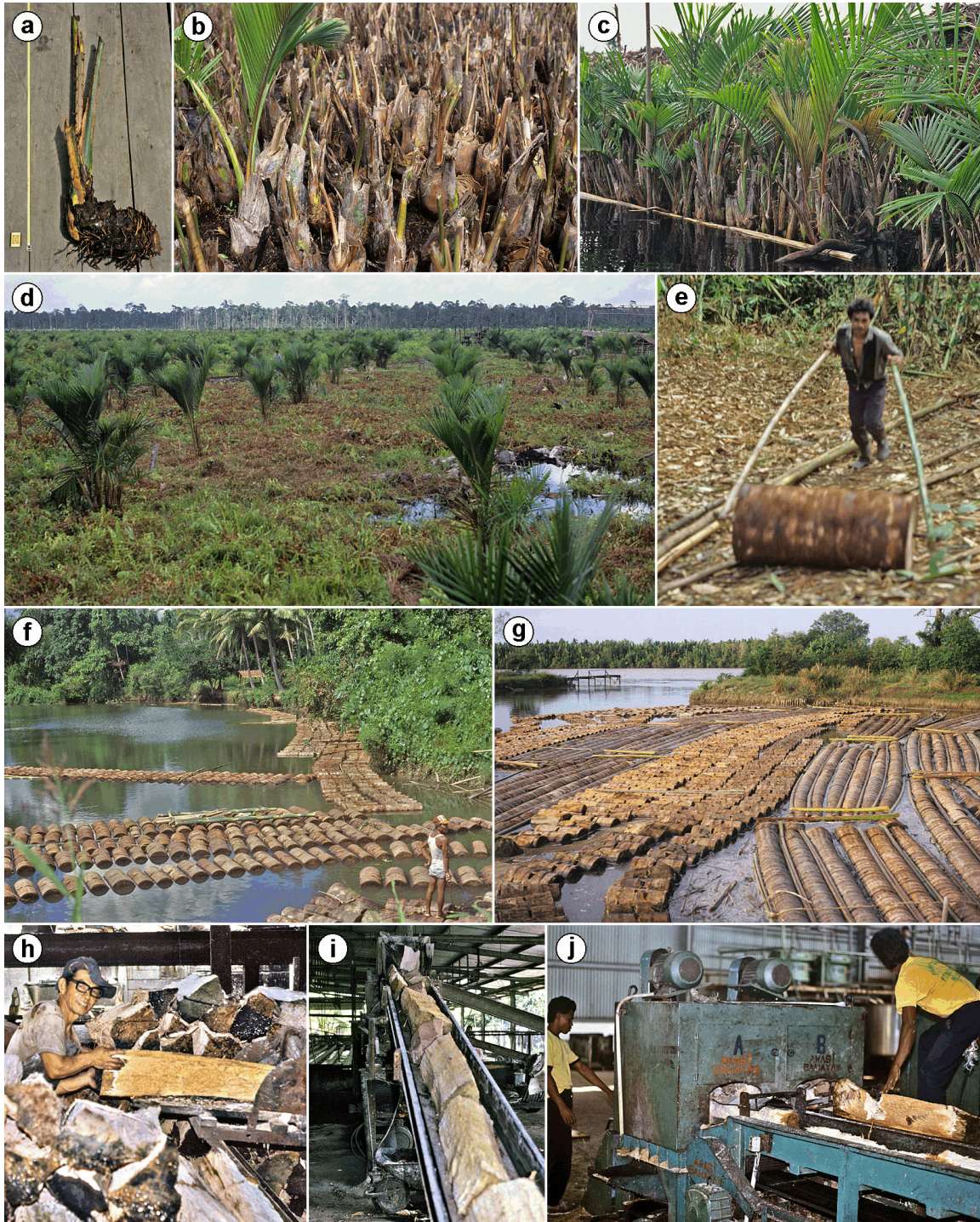
Figure 2.9 Estate cultivation of sago palm and centralised mechanical processing of trunks.
