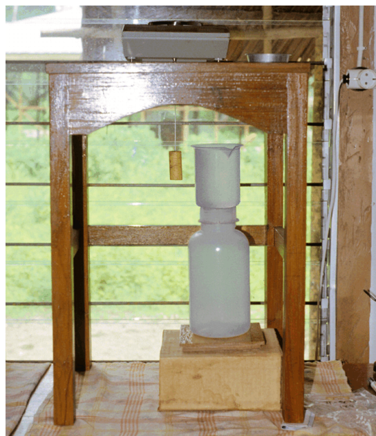
Figure 7.3 Set-up for sample volume measurement by under-water weighing. The balance is placed on a small table with a hole in the top. [photo nr. 89.08-094-18, field lab, Hatusua mon21aug1989]
