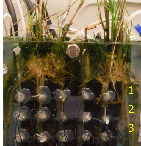
Figure 4: Long term current generation in \text{mA m}^{-2} PGA, Left: Average current generation of each of the 30 anodes from day 102 to day 115 at an anode potential of 50 mV. Right: Photo of the shoots and roots of the plants on day 130. Numbers show the layers of anodes
