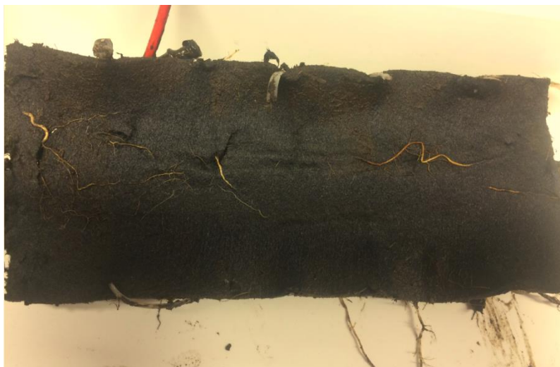
Figure 6: Roots are growing through the anode felt of peat soil PMFC1. Picture from the inside of the anode felt of the dismantled peat soil PMFC1 at end of experiment
