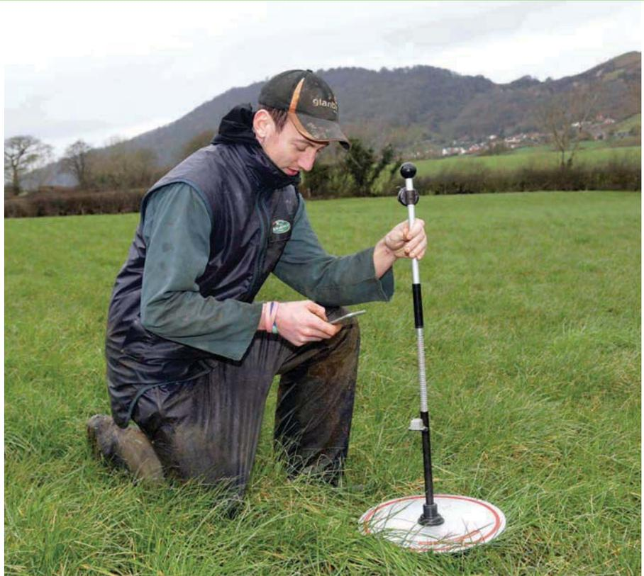
Measure and monitor: a plate meter is used to check on grass growth at least once a week
