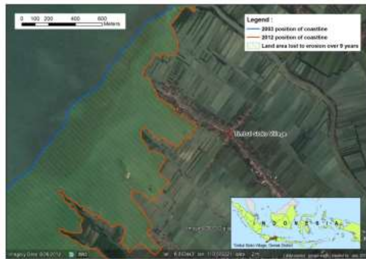
Figure 2.1 Example of coastal erosion in Demak district near Timbul Sloko village, illustrated through the coastline in 2003 (blue) and in 2012 (red).
