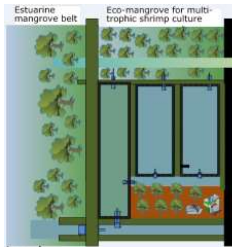
Figure 4.7: Design of a mixed mangrove-aquaculture system, maintaining mangroves ecosystem functions and allowing to optimise shrimp production (Bosma et al, 2014). Black = road, brown = homestead, dark green = earthen dikes, light green = 'green water' pond, clean water indicated in blue and waste water in green.
