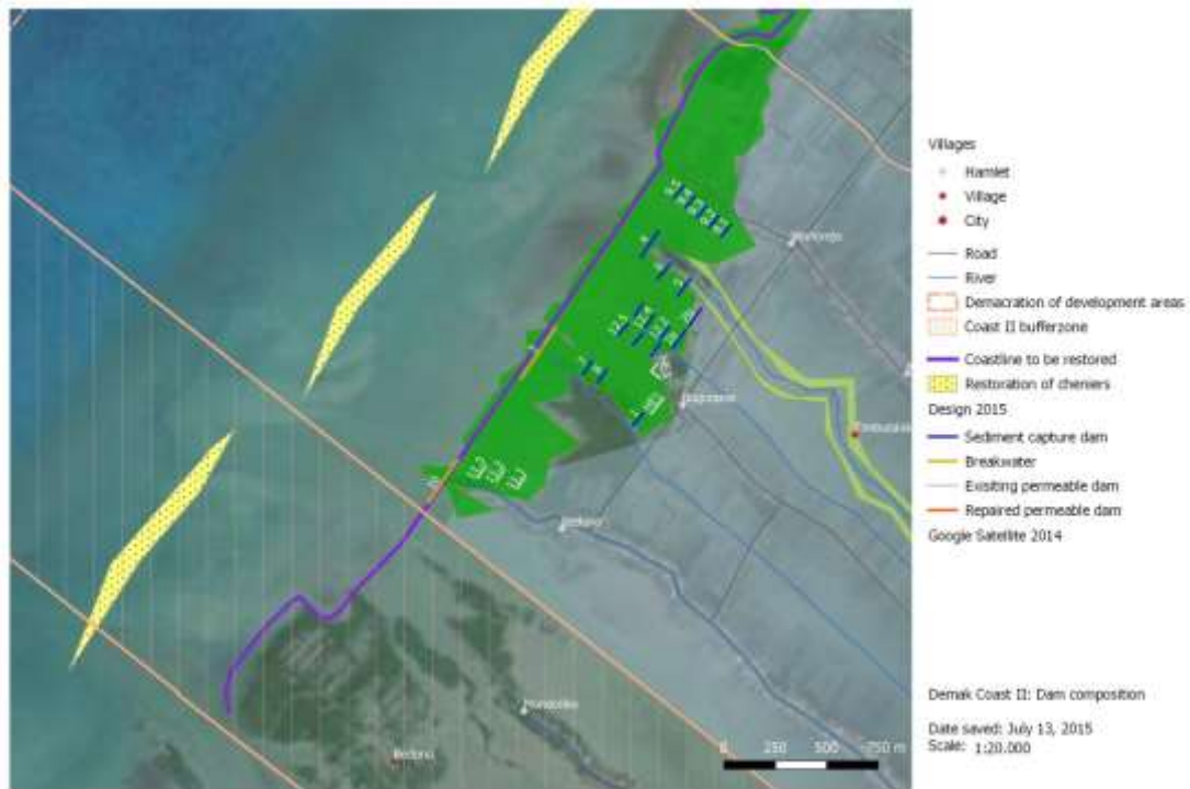
Figure 5.5. Spatial design of coastal safety measures in Coast I/II planned for 2015, in collaboration with MMAF.
