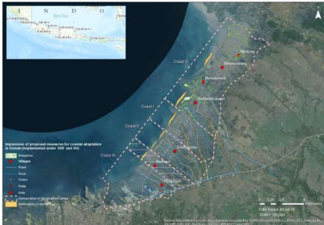
Figure 2.6. Zonation of project area on the basis of severity of erosion and subsidence as well as aquaculture practice.
