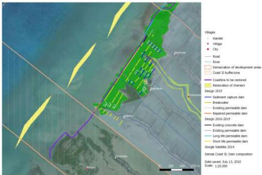
Figure 5.4. Tentative (!) spatial design of coastal safety measures in Coast III for 2015 – 2019, to be achieved by multiple stakeholders as aligned in a Masterplan.
