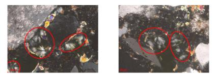
Figure 5.9: Examples of the studied thin sections under the polarized light with the highlighted ettringite (Po6 and Po2).
