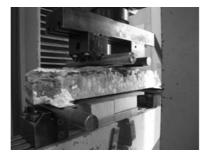
Figure 5.2: Test set-up used for four-point loading flexural tests.
