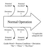
Figure 2.1: Schematic diagram of the HAZOP analysis.
