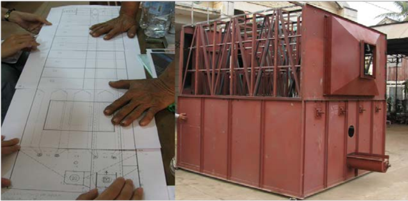
Photo 4.7: Initial design by a miller from Pursat of a recirculating-batch dryer (left); a unit manufactured for another miller (right); Photo by R.Flor
