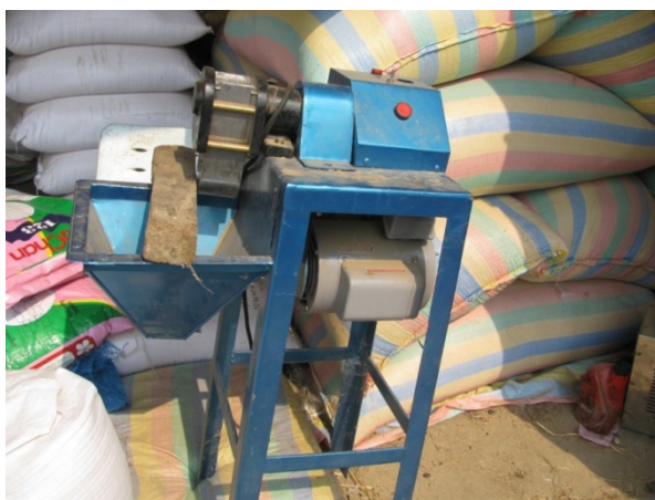
Photo 4.9: Small milling machine: Testing tool used by millers to know purity of grains; also indicates if grain is well dried (not chalky, not easily broken); Photo by R.Flor
