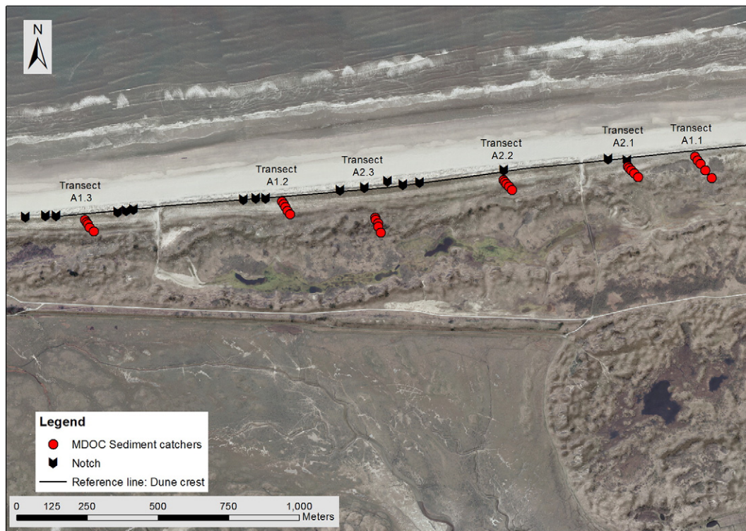
Fig. 3. Aerial photo underlain by digital elevation map of the study area with location of the six transects. Transects A1.1, A1.2, and A1.3: intact foredune. Transects A2.1, A2.2, and A2.3: foredune with a notch cut into it. MDOC = marble dust collector.
