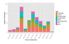
Figure 1. Distribution of the year of construction of bridges and hydraulic structures in The Netherlands.
