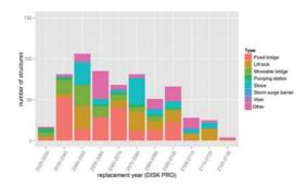
Figure 5. Distribution of the replacement year of bridges and hydraulic structures (DISK PRO).
