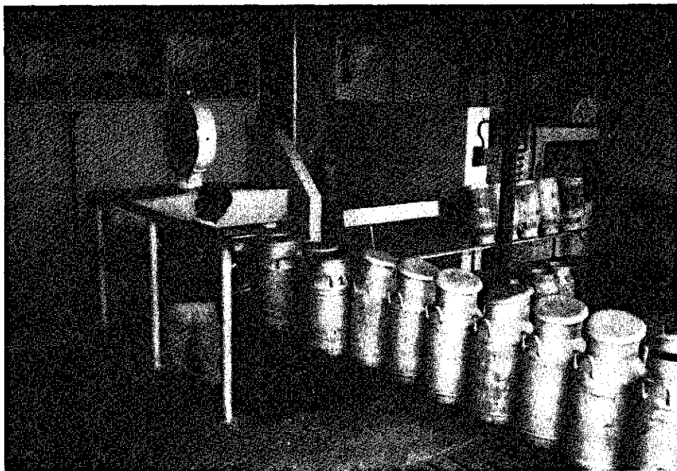
Fig. 21. Milk reception. A roller conveyor transports cans of milk to the scales, where the milk is weighed. After emptying, the cans are put upside down on a drainage rack within reach of the rotary can washer in the background (on the right). Photo: M.A. Luijkx.
