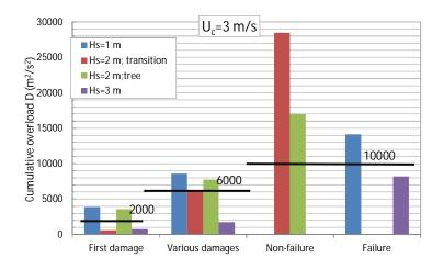
Figure 4.1 Comparison of cumulative overload for various damage thresholds;  $U_c = 3 m/s$
