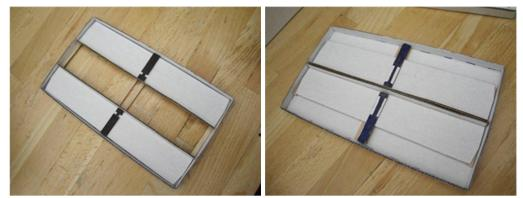
Figure 2.1. Drawer type valve mechanism (open left, closed right)
