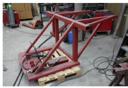
Picture 14 Frame for transport of modules
