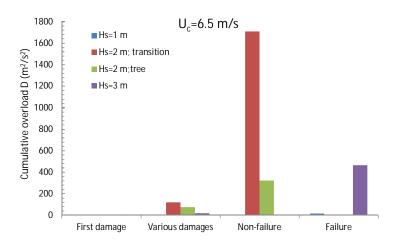
Figure 4.5 Comparison of cumulative overload for various damage thresholds;  $U_c = 6.5 \text{ m/s}$
