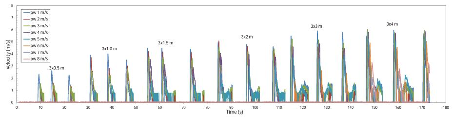
Figure 2.16a. Measured record of flow velocities for filling levels from 0.5 m to 4 m.
