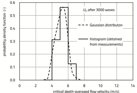
Figure 7.10 Probability function of the critical flow velocity (based on turf-tensile tests)
