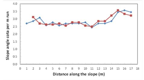
Figure 2.3. Inclination of the dike slope (cota) measured every m along the slope
