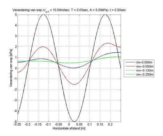
Figure 6.14 Fluctuating pressure as function of time; front velocity is 10 m/s
