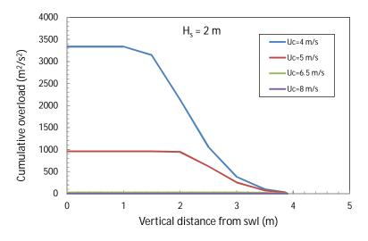
Figure 8.4. Cumulative overload as a function of location on the seaward slope, for  $H_s = 2 m$
