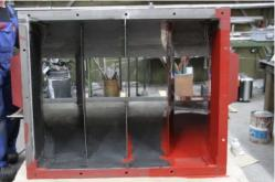
Picture 12. Inner part with guiding plates
