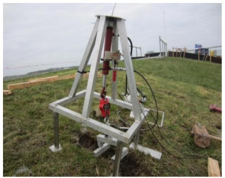
Figure 7.4 Turf-tensile apparatus (pull frame is inside the apparatus)
