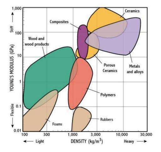
*Figure 7.11* Young's modulus as function of the density for various materials (source: <u>http://www-materials.eng.cam.ac.uk/mpsite/interactive\_charts/stiffness-density/NS6Chart.html</u>)
