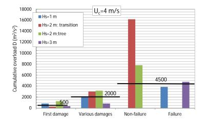
Figure 4.3 Comparison of cumulative overload for various damage thresholds;  $U_c = 4 m/s$
