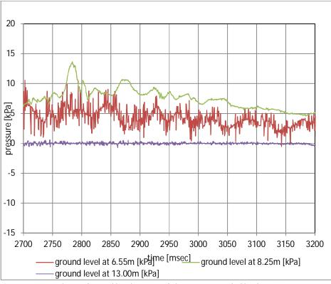
Figure 6.9 Location p2 (ground level at 8.25 m) the pressure period is about 30 msec
