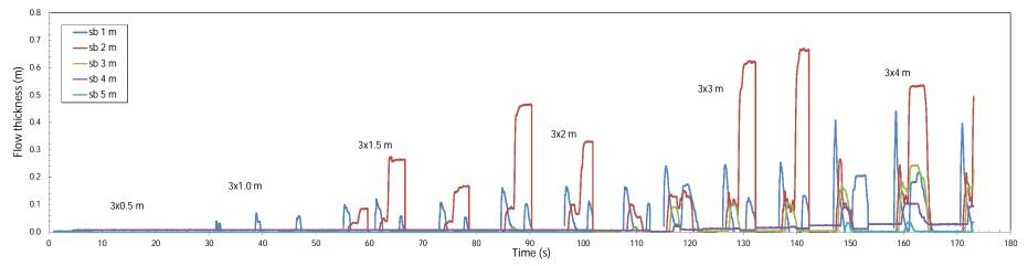
Figure 2.16b. Measured record of flow thicknesses for filling levels from 0.5 m to 4 m
