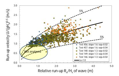
Figure 8.2 Run-up velocity (maximum) versus relative run-up level
