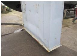
Picture 35. Bended lower module water column
