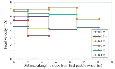
Figure 2.23. Front velocities as a function of the distance along the slope
