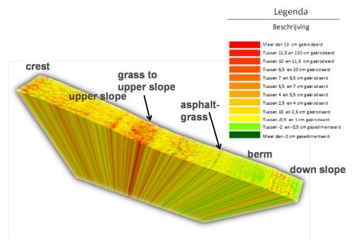
Figure 5.1. Measured erosion for test 1
