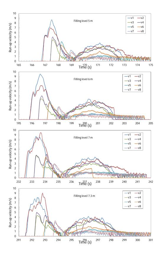
E Measurements of velocity and flow thickness along the slope during the hydraulic measurements at the Zeelandbrug and for various filling levels
