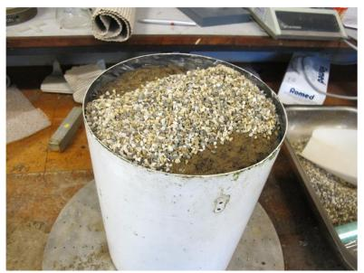
Figure 6.11 Preparing the bottom side by picking off clay parts and application of gravel layer
