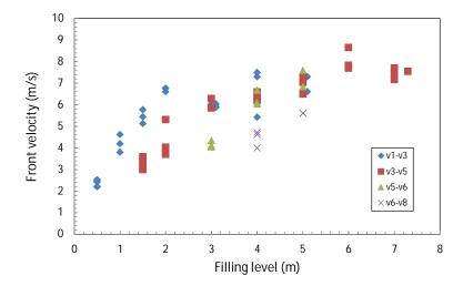
Figure 2.22. Front velocities as a function of the filling level
