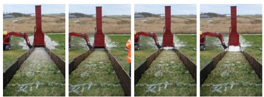
Figure 12. The run-up process for a filling level of 6 m.
