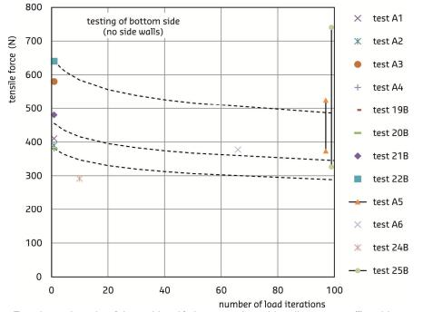
Figure 7.8 Experimental results of the rapid and fatigue tests (two sidewalls were cut off) rapid tests after one load cycle; fatigue tests after about 100 load cycles
