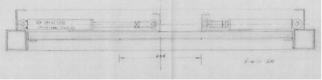
Figure 10 Adjustable leg of frame
