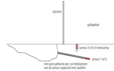
Figure 6.3 Pressure sensors
