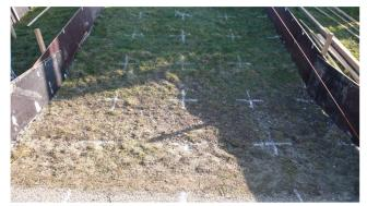
Figure 5.9. Quality of the grass berm was bad at Tholen (before testing)
