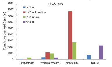
Figure 4.4 Comparison of cumulative overload for various damage thresholds;  $U_c = 5 m/s$
