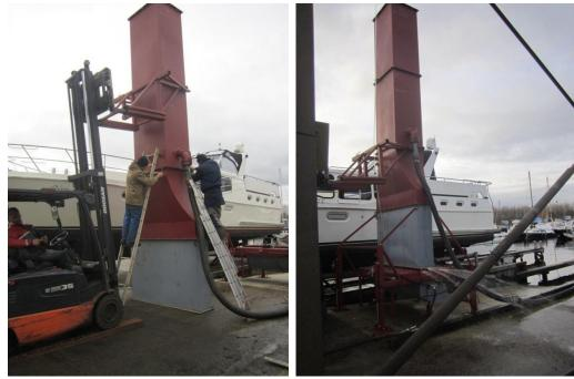
Picture 31. Fixing for 7 m water column testing
