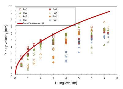
Figure 2.19. Maximum run-up velocities along the dike section
