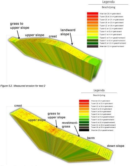
Figure 5.3. Measured erosion for test 3
