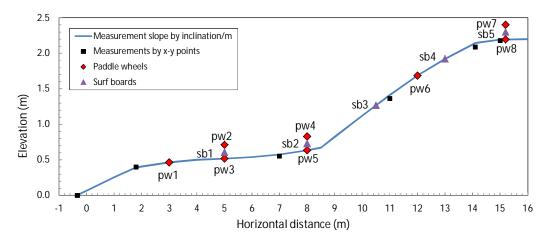
Figure 2.15. Geometry of the dike for hydraulic measurements and locations of instruments
