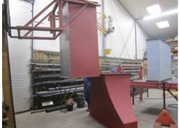
Picture 17. Placing upper box on transition
