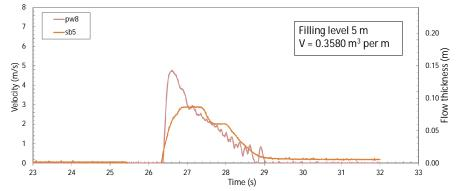
Figure 2.25. Flow velocity and thickness at the crest for a filling level of 5 m
