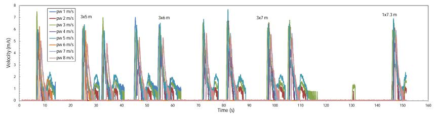
Figure 2.16c. Measured record of flow velocities for filling levels from 5 m to 7.3 m
