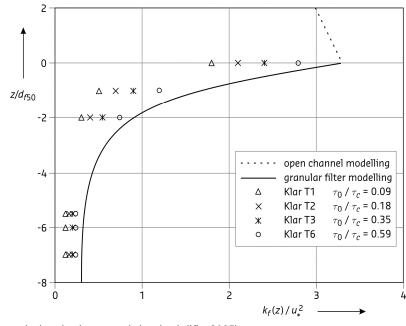
Figure 6.2 Dimensionless load versus relative depth (Klar 2005) ( $\tau_0$  is the bed shear stress and  $\tau_c$  is the critical bed shear stress)
