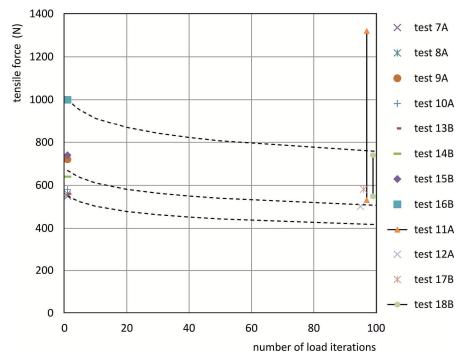
Figure 7.9 Experimental results of the rapid and fatigue tests (two sidewalls were cut off) rapid tests after one load cycle; fatigue tests after about 100 load cycles
