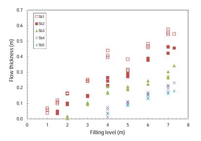
Figure 2.20. Maximum flow thicknesses along the dike section
