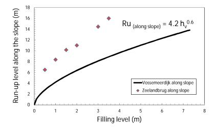
Figure 2.13. Measured run-up along the slope as function of filling level for the Vossemeerdijk and section 1 at the Zeelandbrug
