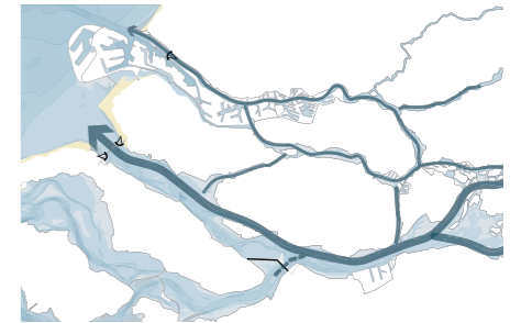
Figure 6.26 Most river discharge via the Haringvliet
