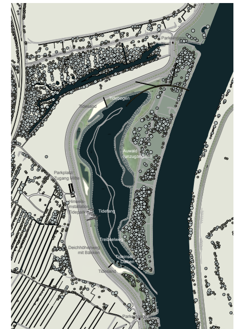
Figure 9.15 Design of the Kreesand Tidal Park riverbed widening project (Hamburg Port Authority, Studio Urbane Landschaften Hamburg / OSP)
