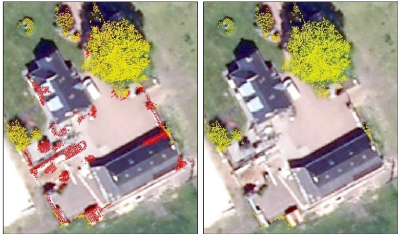
Figure 62: Part of the study area where NDVI (right image) is applied to remove misclassified non-vegetation points (red dots in left image)
