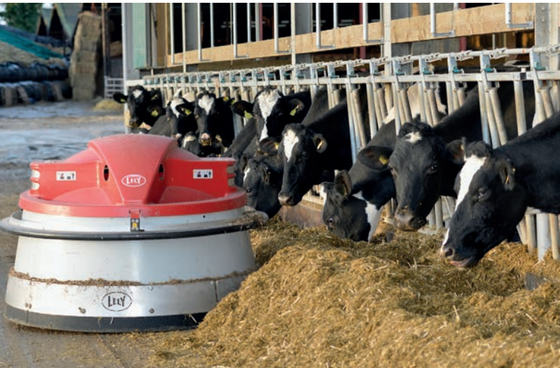
Helping hand: a robot pushes feed up to the barrier every two hours
