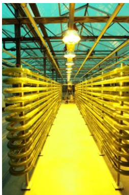
Figure 6: Picture of the airlift reactor used for cultivation [15]
