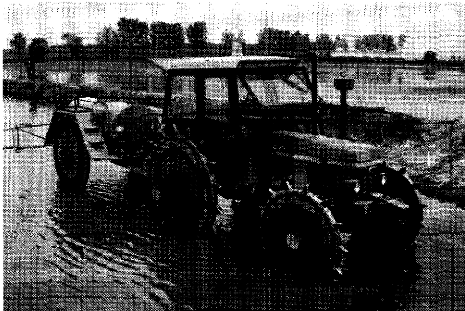
Fig. 2 - Herbicides and other pesticides are applied using trailed sprayers fitted with smooth, large diameter, narrow, steel wheels.
