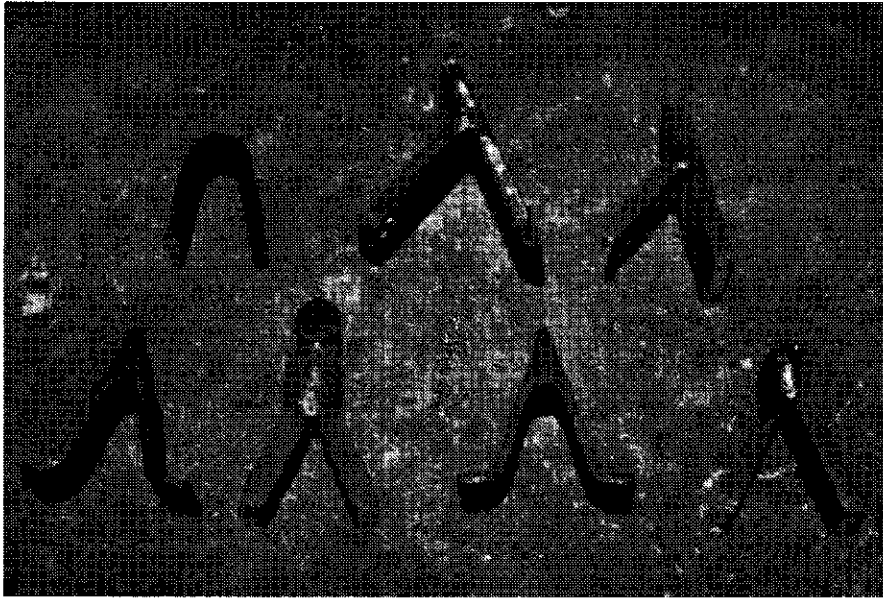
Fig. 4 - A wide range of lug shape and size equipping narrow steel wheels can be found, selected by farmers in order to minimize wear, rather than to improve tractive performance.
