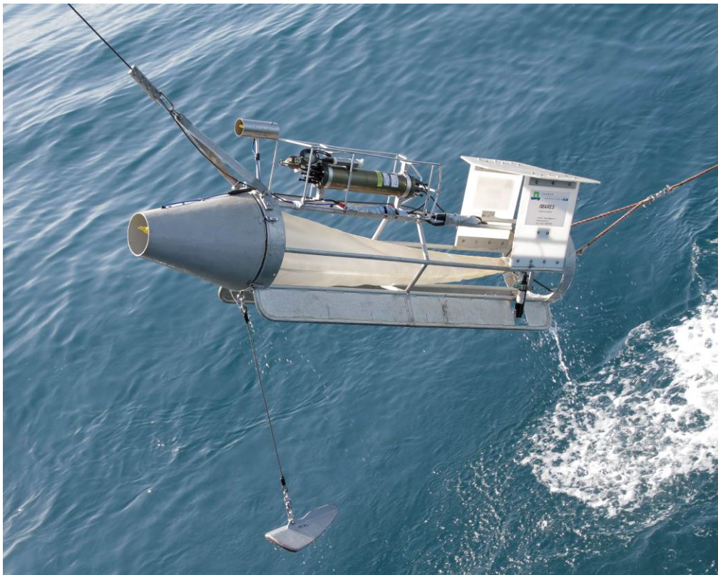
Figure 3.1. Gulf VII high speed plankton sampler.
