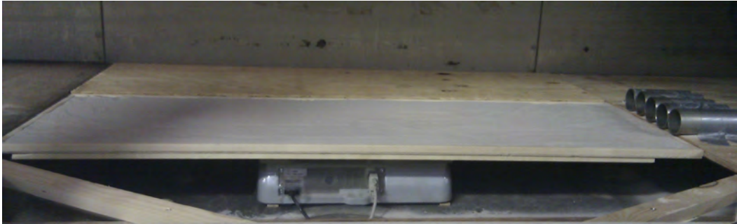
FIGURE 4.3: Image of the experimental setup. The balance was placed underneath the test tray in order to measure the weight of the sediment throughout the experiment. The image taken during the calibration, when the five saltiphones were placed next to each other.
