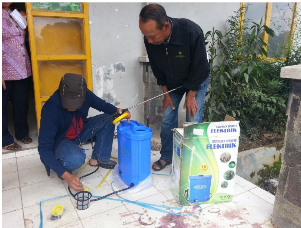
Photo 3. A battery powered knapsack sprayer was used in both demo-plots in Garut and Pangalengan.
