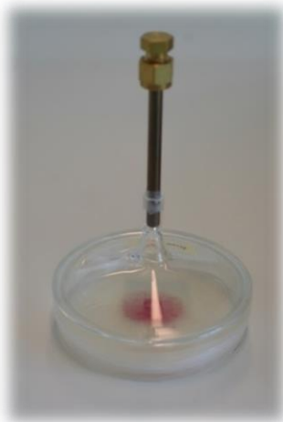
Figure 2 Petri dish with special lid containing the volatile trap. (photo Ruth Schmidt)
