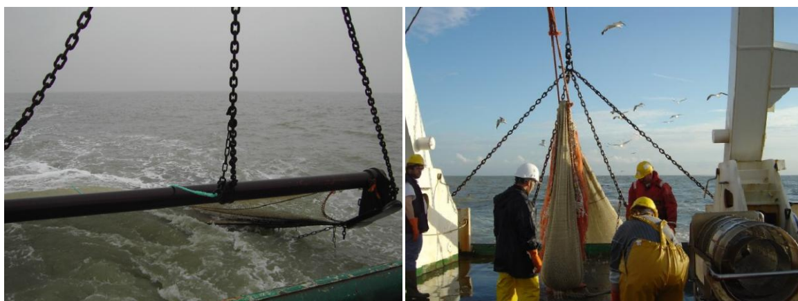
Figure 13. An 8-meter beam trawl with a fine-meshed shrimp net and a bolder chain.
