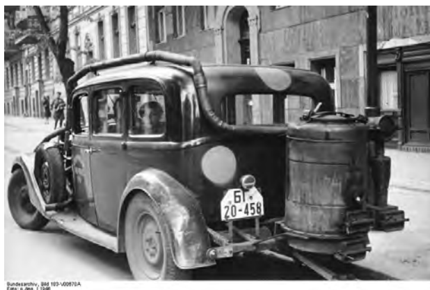
Figure 6.2: One out of more than 750.000 wood gas vehicles in Europe at the end of the Second World War that used fuelwood due to rationing of fossil fuels (Anonymous, 1946).
