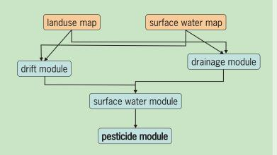
Components of the CASCADE model to predict pesticide exposure concentrations in a network of watercourses.
