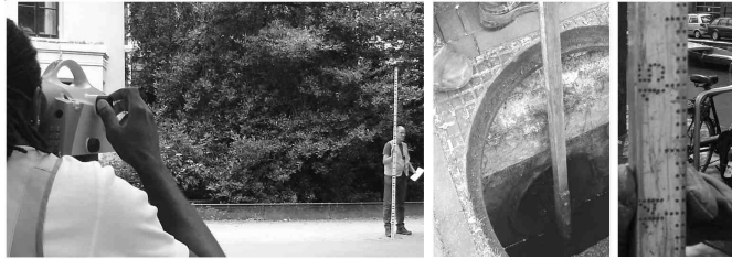
Figure 3.3: Left: measurement of a manhole cover using a levelling instrument. Middle: measurement of the distance between invert level and manhole cover using a rod. Right: graduation on the rod.
