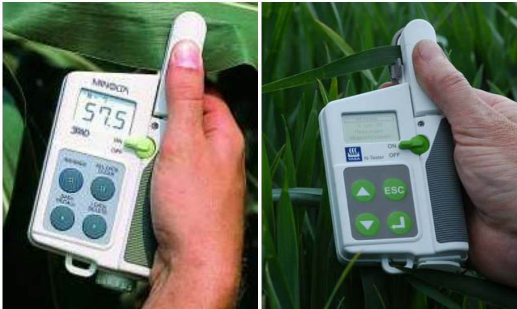
Figure 5: SPAD-502 chlorophyll meter and N-tester (Photos taken from The Garden Professors™ blog and Agri Con website respectively)
