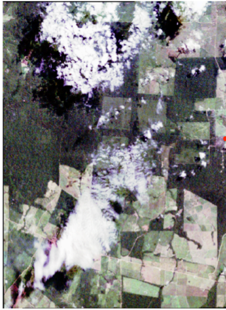
Fig. 5 An example of the validation procedure. A validation sample (in red) is plotted over a True Colour composite of the study area based on Landsat Surface Reflectance products (date: 2008-06-27). The composite is created with bands 3, 2 and 1 in R software.
