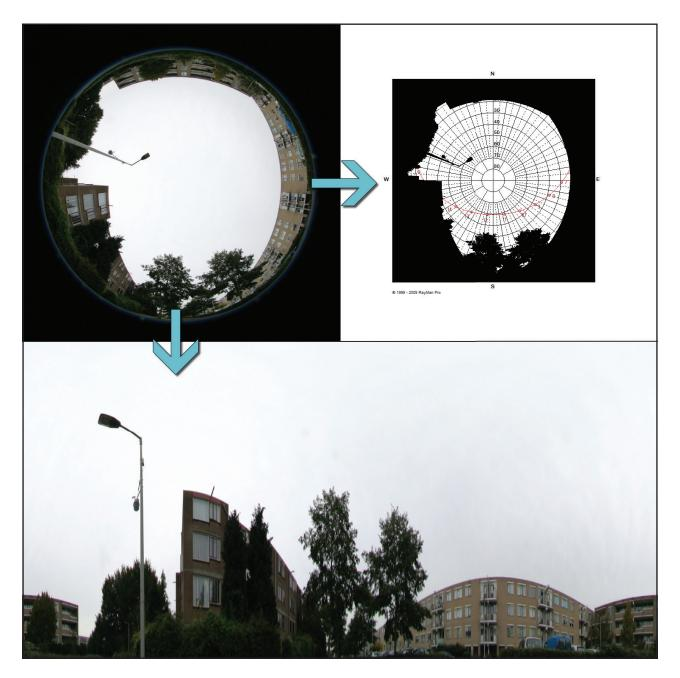
Figure 5: Original fish eye photograph of station #Ams4 (Top left), the transformation used to calculate Sky view factor and incoming solar radiation (top right) and a panoramic transformation (bottom).
