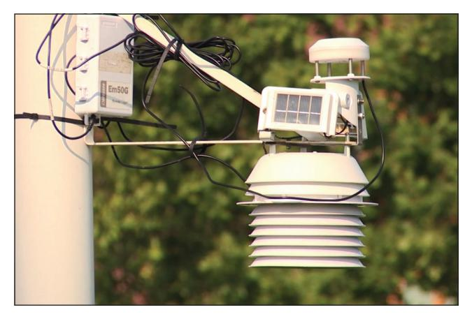
Figure 3 Setup of a weather station as used in this research. Wind measurements are performed in the cylinder on top, temperature and humidity is measured in the larger cylinder below the solar panel. a datalogger is attached to the pole on the left.
