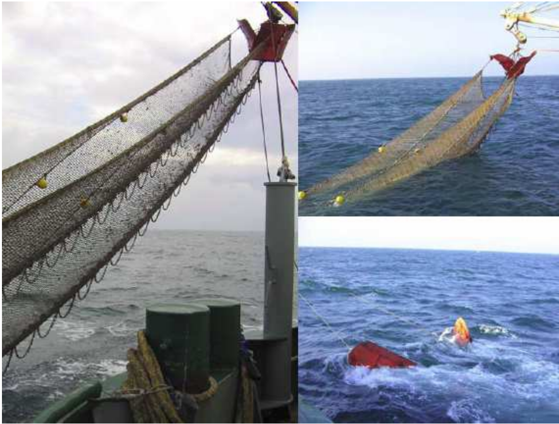
Figure 5-7: Outrigger system used on Dutch beam trawlers in 2006.
