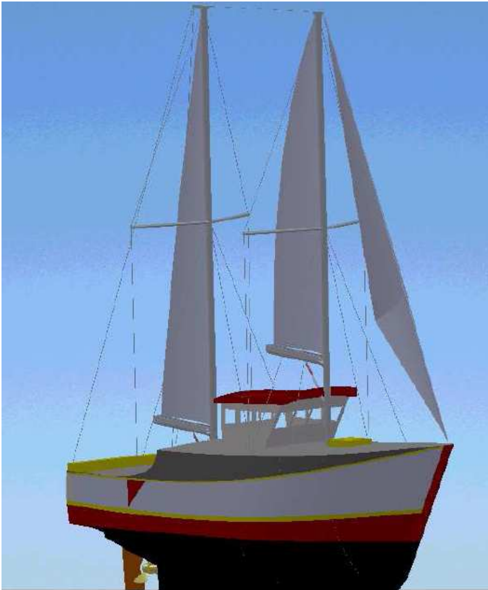
Figure 5-49: Primary sketch of trawler equipped with automatic sail propulsion system.
