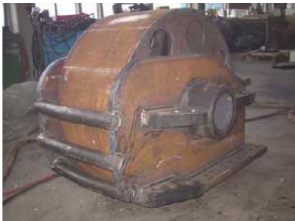
Figure 5-1: Wheel to replace beam trawl shoe
