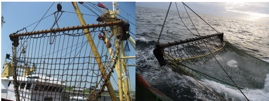
Figure 3: Chain matrix beam trawl (rigged with roller gear (left), shooting (right))
