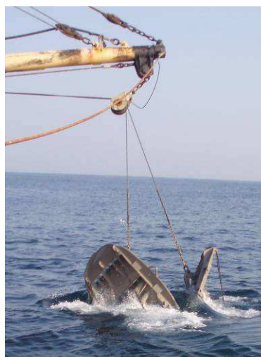
Figure 5-11: Launching the otter boards from the derricks
